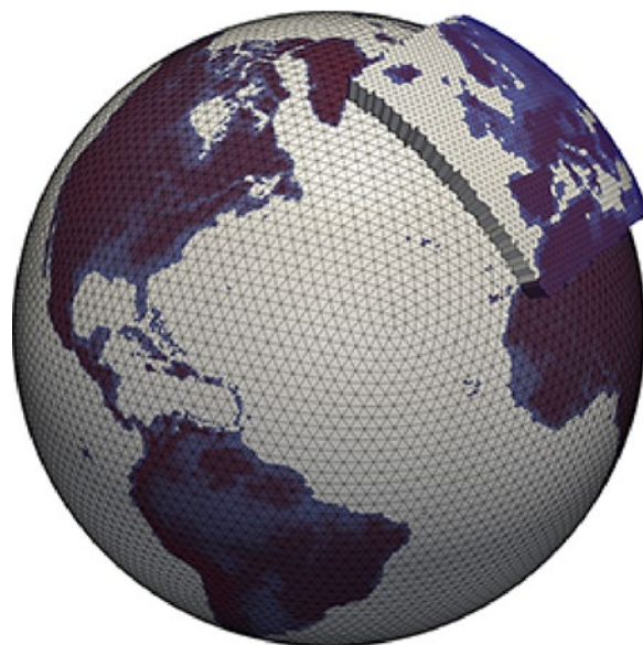
Figure 2.22. Schematic depiction of an icosahedral grid with regional refinement over Europe as implemented at the German Meteorological Service ( Deutscher Wetterdienst )
