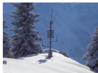
BELOW: A typical measurement site for SWE, LWC and snow depth measurement
